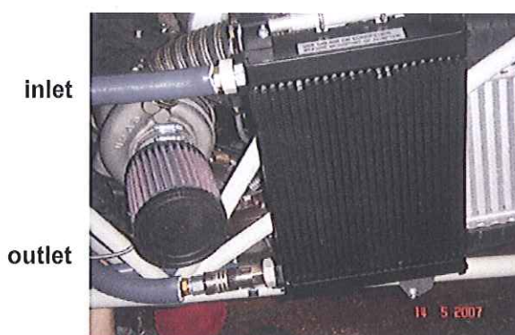
Fig. 1 new oil cooler (inlet is positioned at upper side and outlet at lower side of cooler)
